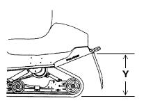
To determine sag, commonly referred to as ride-in, subtract measurement Y from X (sag=X-Y). Adjust sag by rotating the torsion spring preload cams located on the rear torque arm. Use the illustration for reference. The ideal amount of Sag for the EDGE rear suspension is four inches (X-Y=4).
